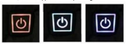
To turn off the heating of the vest, it is necessary to press the switch for 3–5 seconds.
